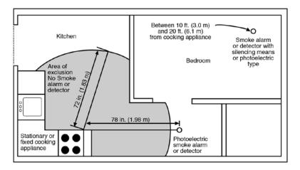
Photoelectric devices may be installed up to six feet from a fixed cooking appliance.
