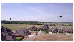
xCraft's x2i Hybrid VTOL drone, which runs on Rajant's InstaMesh networking technology, and can fly for 45 minutes at speeds up to 60 mph. The tests proved that a home alarm company can get aerial surveillance on the scene as quickly as 30 seconds.
